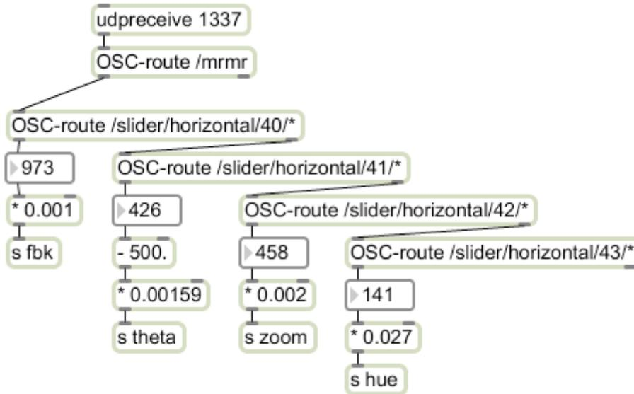
Figure 18. iPhone control of feedback via mrmr.
