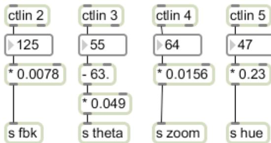
Figure 17. Midi based feedback control patch.
