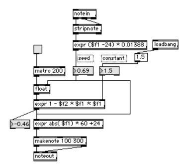
The main calculation takes place in [expr 1-\$f2 \* \$f1\*\$f1]. The other two expressions scale the input and output to appropriate values. Deriving the seed from note in gives a nice performance feature. Each key produces a unique
