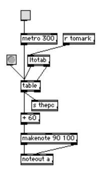
I've used send and receive objects to make it easy to connect a graphic front end. (That front end is presented in User Interface Design in Max). In this instance we'll use a coll:
