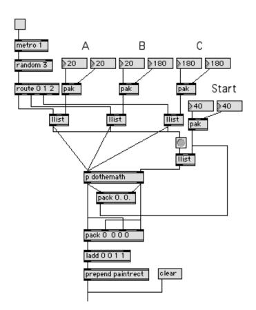
The bottom lines go to the LCD. You can see how the three corners and the starting point are entered. The metro will make the plotting fast enough to watch the process. Here's how new points are calculated:
