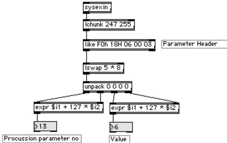
The format for the return message is F0 18 06 id 03 pl pm vl vm F7, where pl and pm give the parameter number as before, and the vl and vm are the current value. The Like object will pass lists that start with the arguments<sup>4</sup>. Like also recognizes hex in the 00h format, and will consider any other symbol a wild card,
