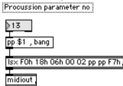
There are two common ways that instruments refer to data, one is by direct memory addressing, the other is via parameter numbers. The Procussion uses parameter numbers, which you get by reading the documentation. Then the message F0 18 06 id 02 pl pm F7 will cause Procussion to return the current value for the parameter. The bytes in that message mean:
