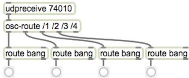
Figure 11. Detecting tab changes.
