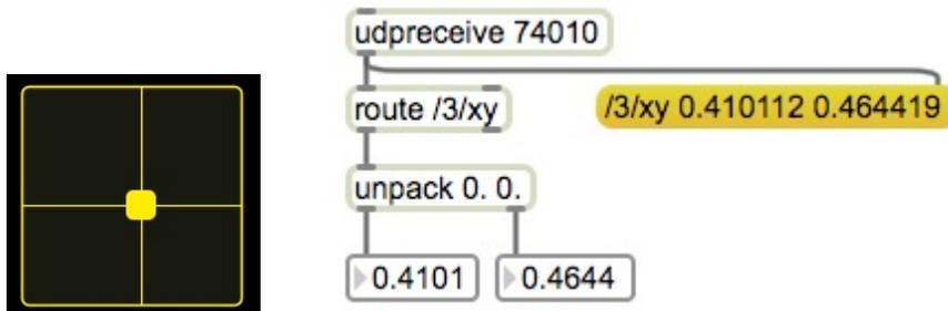
Figure 12. Unpacking XY.
