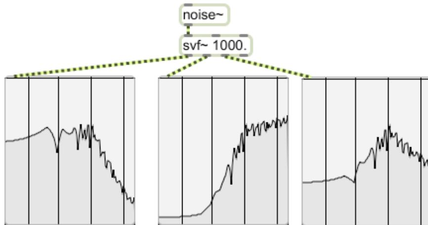
Figure 9. Low pass, high pass and band pass outputs of svf~
