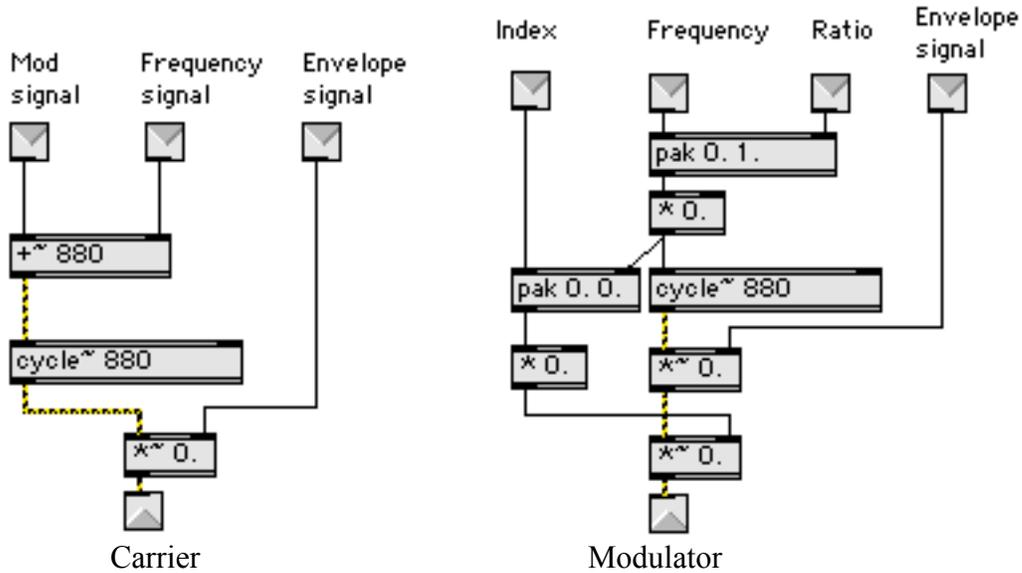
Figure 11. Subpatches of Fig 10.
