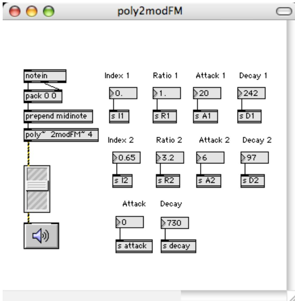
Figure 14. A complete FM instrument
