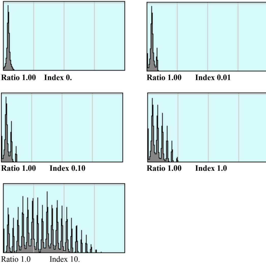
**Figure 3. Effect of modulation index**
