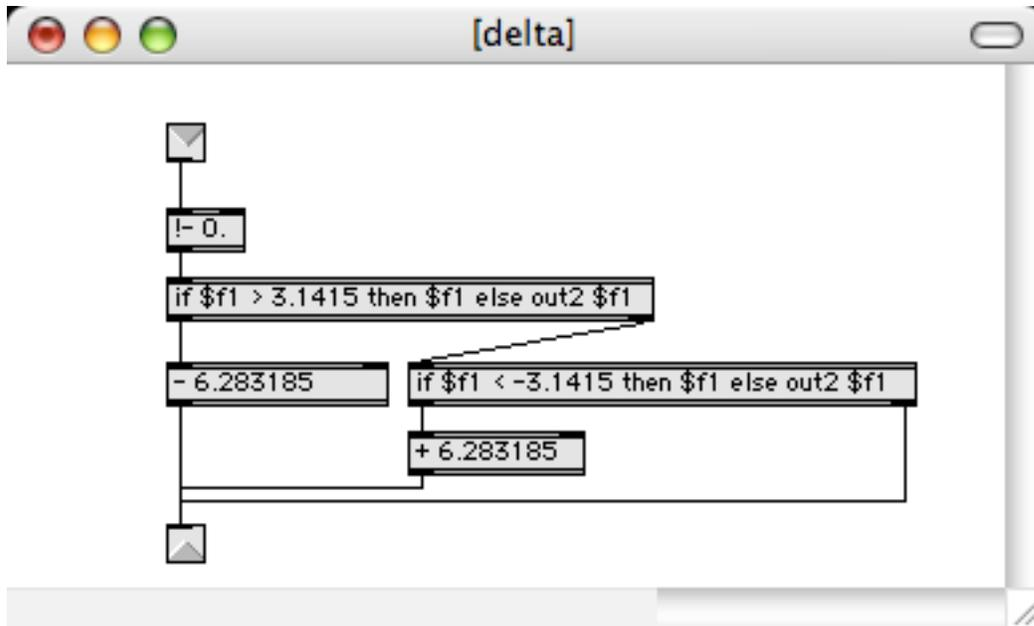
Figure 5. Fixing the angle wrap problem.
